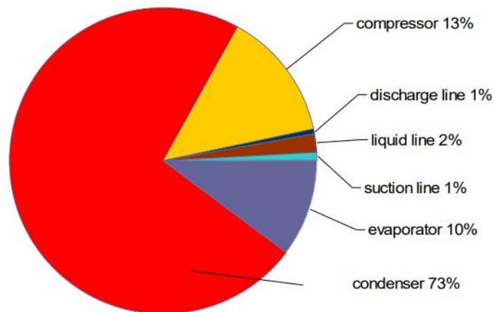
Figure 2. Typical refrigerant charge distribution in an AC system
