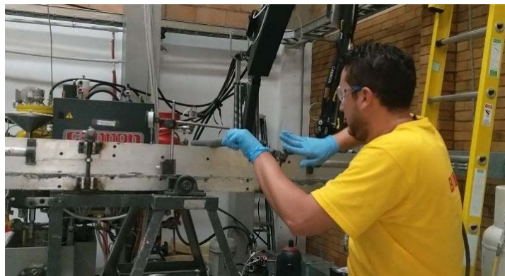
Figure 5. Measurement of foam expansion at Brett mould
