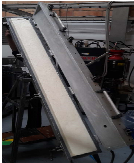
Figure 4. Determination of Minimum Fill Density (MFD)
