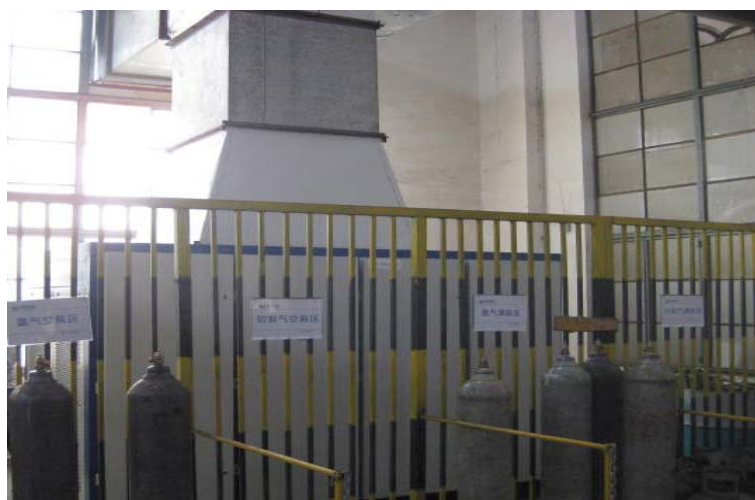
Fig 9. High pressure test equipment for CO2 vessel
