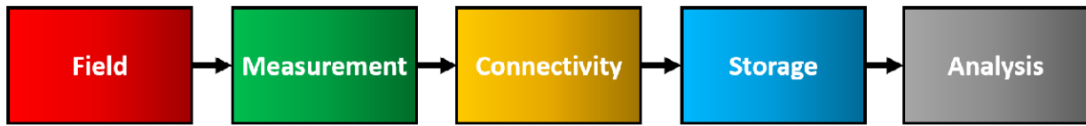
Figure 1 Flow chart of digital data collection (source: IIR, 55th Informatory Note on Refrigeration Technologies, 2023)
