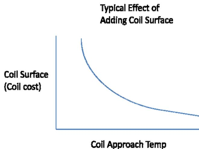
The approximate range of coil approach temperatures for evaporator and condenser coils is between 20 °F (1 row smooth bore tube coil) to 10 °F (4 row IE tube). 10 °F is nearly a practical limit.
